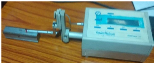
Fig. 3. Surface Roughness Measurement Instrument (Taylor Hobson Subtronics3+)
