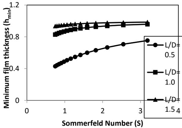
Fig. 5: Minimum fluid-film thickness versus Sommerfeld number
