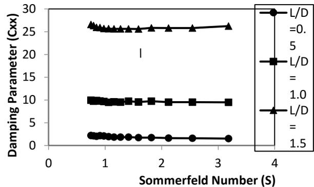
Fig.12: Direct fluid-film damping coefficient versus Sommerfeld number
