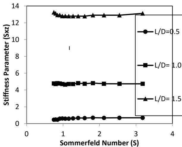
Fig. 10: Cross-coupled fluid-film stiffness coefficient versus Sommerfeld number
