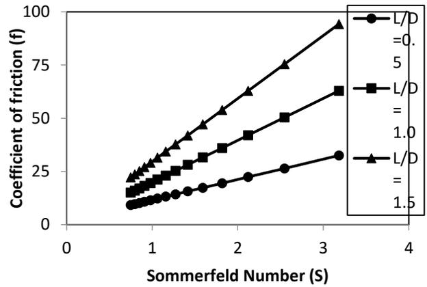
Fig. 7: Coefficient of friction versus Sommerfeld number
