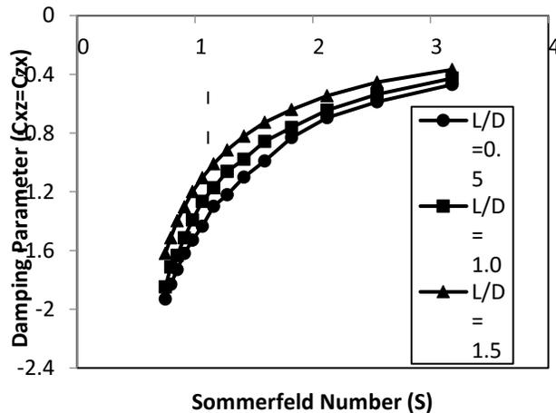
Fig. 14: Cross-coupled fluid-film damping coefficient versus Sommerfeld number
