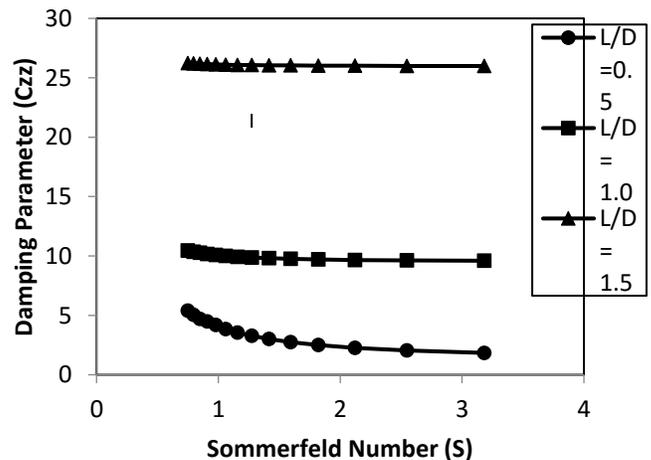
Fig. 13: Direct fluid-film damping coefficient versus Sommerfeld number
