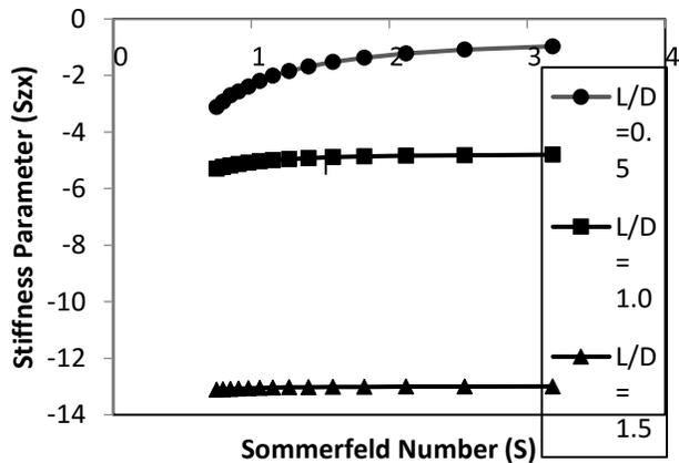
Fig. 11: Cross-coupled fluid-film stiffness coefficient versus Sommerfeld number
