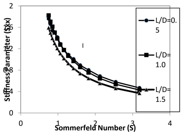
Fig. 8: Direct fluid-film stiffness coefficient versus Sommerfeld number
