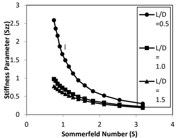
Fig.9: Direct fluid-film stiffness coefficient versus Sommerfeld number
