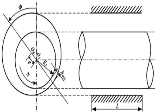
Fig. 1. Definition of the coordinate and the schematic of a simple plain journal bearing.
