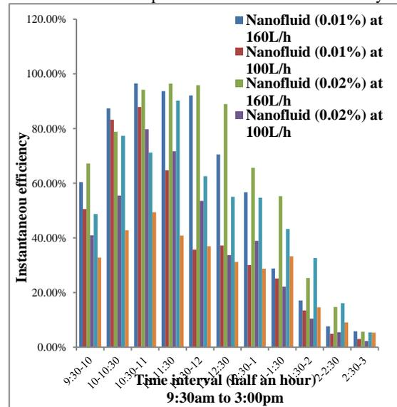
Fig. 2. Experimental variations of instantaneous efficiency [15]
