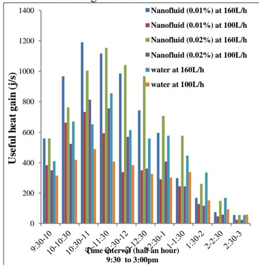
Fig. 1. Experimental variation in useful heat gain by nano fluid and water at different conc and volume flow rates [15]
