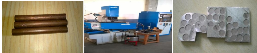
Fig. 1. (a) copper electrodes, (b) EDM setup and (c) machined work piece
