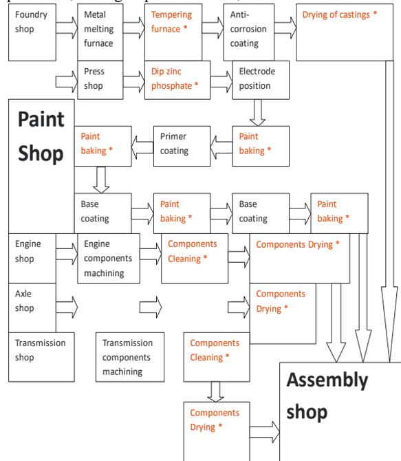
Fig. 6. Different processes needing thermal energy marked in automobile industry
