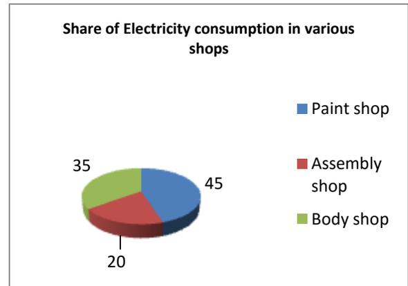
**Fig. 4.** Pattern of Electricity consumption in Different shops in Automobile industry
