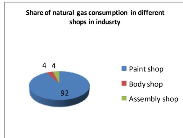
**Fig. 5.** Pattern of Petroleum products (natural gas) consumption in Different shops in Automobile industry
