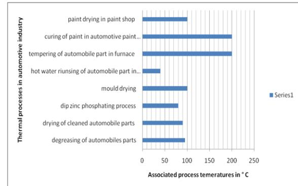
Fig. 7 thermal processes in automotive industry with associated process temperatures
