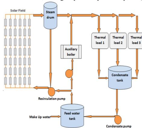
**Fig: 8** layout of the proposed SIPH system for automobile industry
