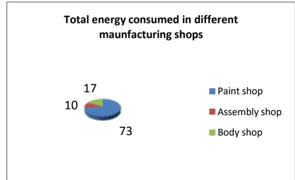
**Fig. 3.** Pattern of energy consumption in Different shops in Automobile industry
