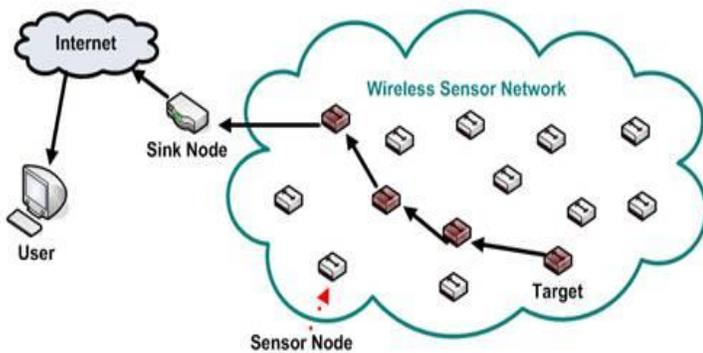
Fig. 1: Conventional Sensor Network
