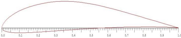
Fig. 2.1 design of Blade
