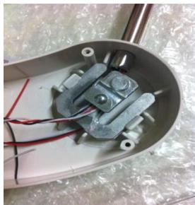
Fig 8: Typical 3 Wire Strain gauge
