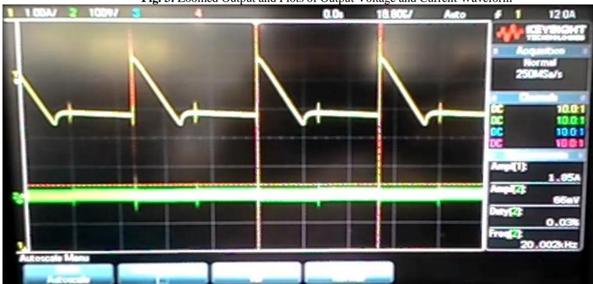
Fig.4 Experimental Output and Plots of Output Voltage and Current Waveform
