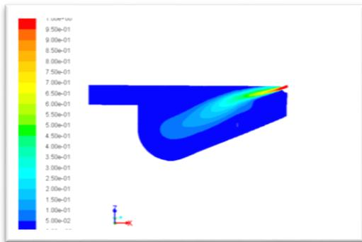
**Fig. 3** Contours of CH4 mass fraction (10° after SOI)
