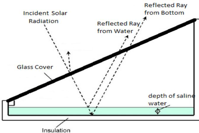
**Fig-1** Schematic diagram of solar still
