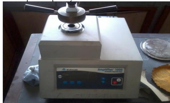
**Fig 3.** Simplimet 100 Automatic Mounting Press.
