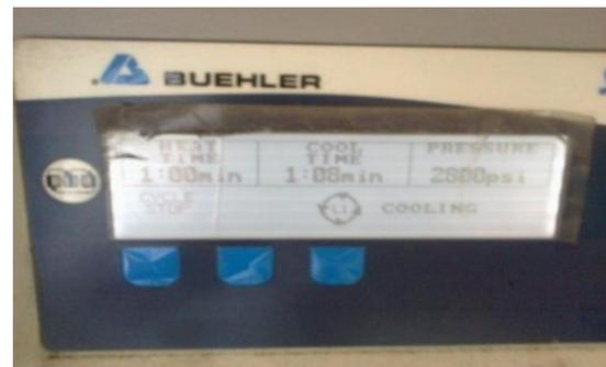
**Fig 4.** Heat time and cool time of Automatic Mounting press.
