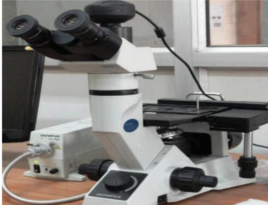
Fig. 6. Olympus GX 41 microscope
