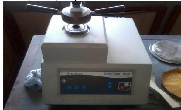
**Fig 3.** Simplimet 100 Automatic Mounting Press.
