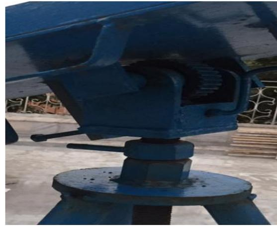
Fig. 1 – Power screw for altering line
