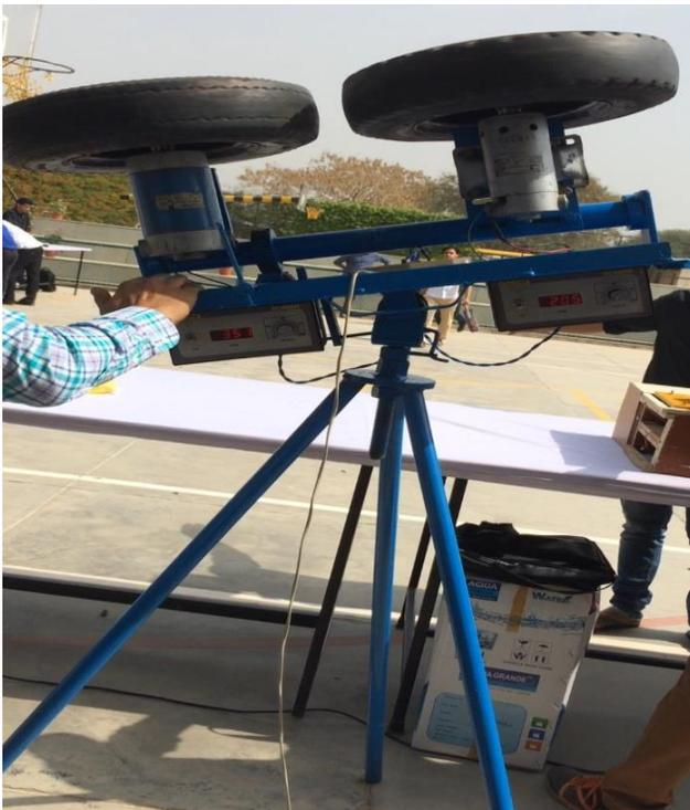
**Fig. 3** – Complete ball projecting machine
