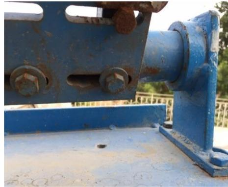
**Fig. 2(b)** – Mechanism to slide motor plate to vary gap between wheels
