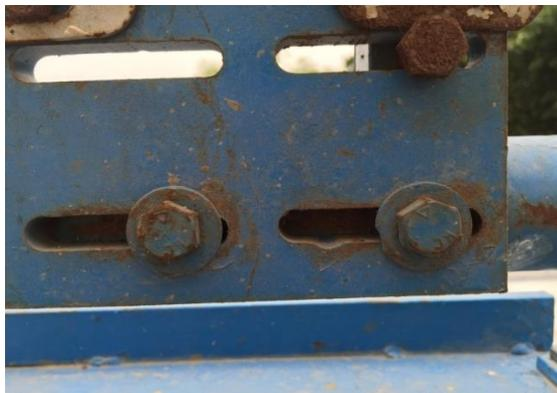
**Fig. 2(a)** – Mechanism to slide motor plate to vary gap between wheels
