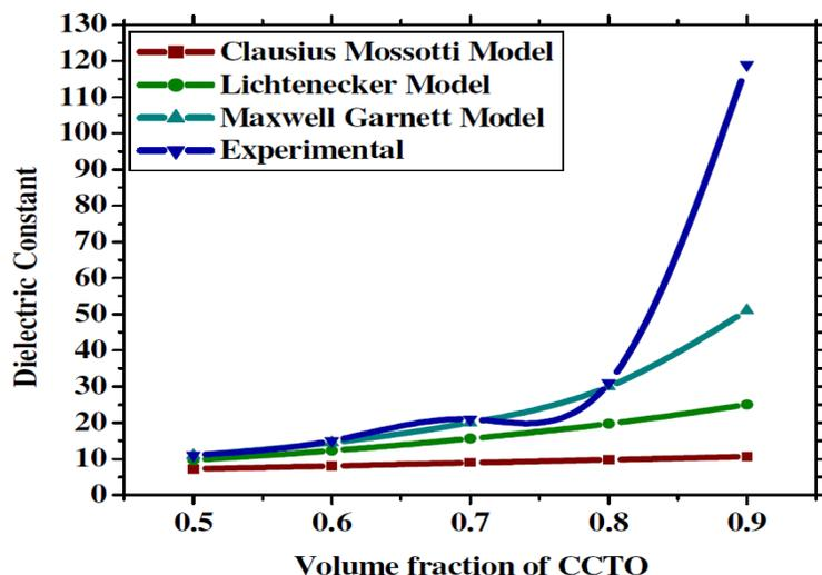
**Fig.5** Comparison of experimental and theoretical dielectric constants of CCTO-silicone resin composites at 1 kHz
