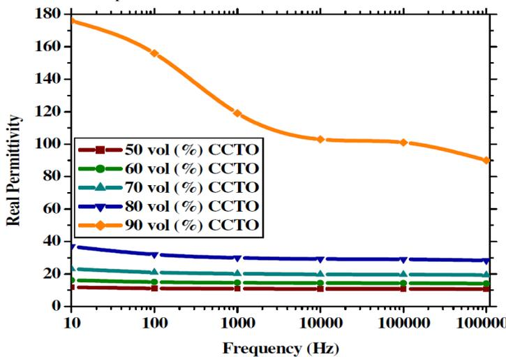
Fig.2 Dielectric constant vs. frequency for composites with different CCTO volume fraction at 30°C temperature.
