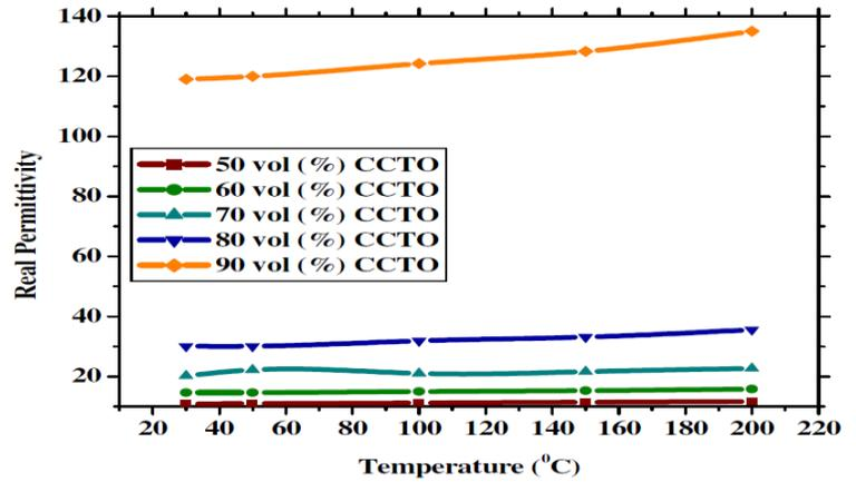
Fig. 3 Dielectric constant vs. temperature for composites with different CCTO volume fraction at frequency  $10^3$  Hz.
