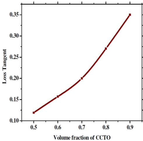
Fig.1 Dependence of dielectric constant and loss tangent of the CCTO-silicone resin composites on the volume fraction of CCTO at 1 kHz and room temperature.
