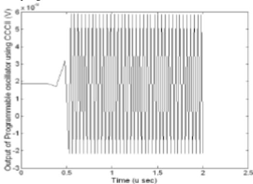
**Fig.6** Output Wave of Oscillator using CCCII. The operating frequency is about 13.16 MHz with  $I_b=800\mu A$ ,  $V_{dd}/V_{ss}=\pm 1.5V$ ,  $C_1$  &  $C_2=1pF$  &  $20fF$ ,  $R_1=1k$ .
