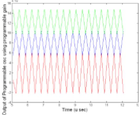
**Fig.7** Output with Programmable Amplitude with CCCII current gain on-chip programming. Output (Red) corresponds to CCCII gain=1.0769, blue corresponds to gain=1.1886 and green corresponds to gain=1.2138.
