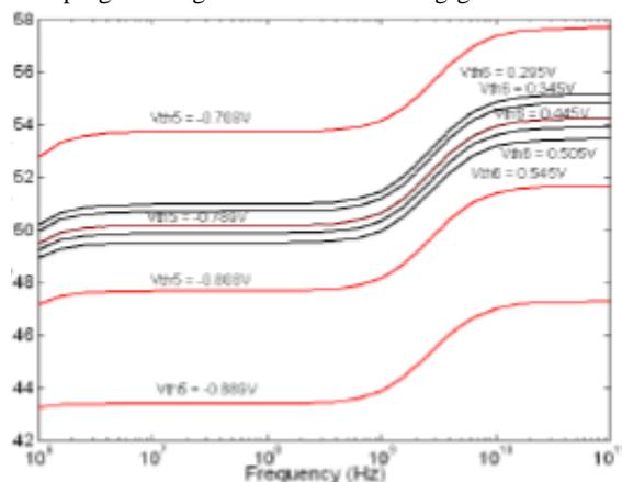
Fig.4 Variation of Voltage gain with change in threshold or programming of M5 and M6 floating-gate transistors
