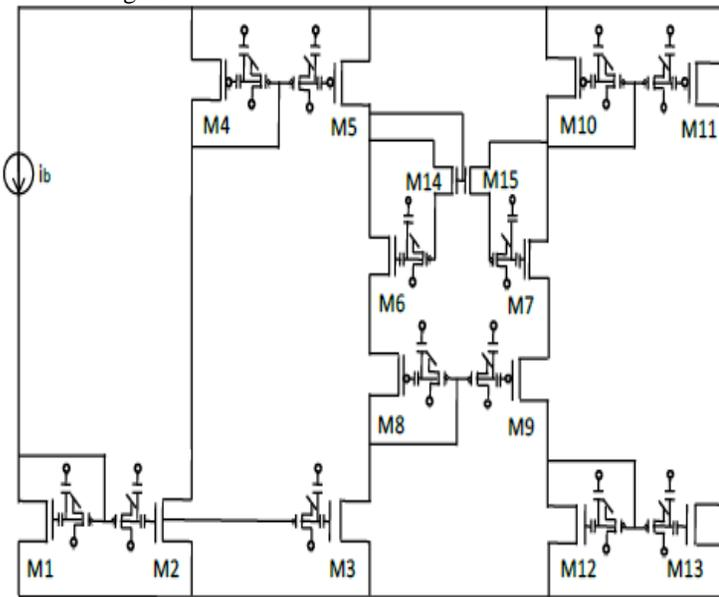
**Fig.1** Proposed CMOS CCCII Design employing programmable FGMOSs
