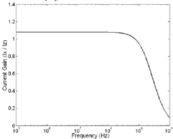
Fig.2 Frequency response of Current gain of CMOS CCCII design with basic circuit configuration
