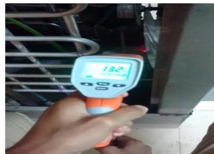
Fig.2 – Infrared Laser gun reading
