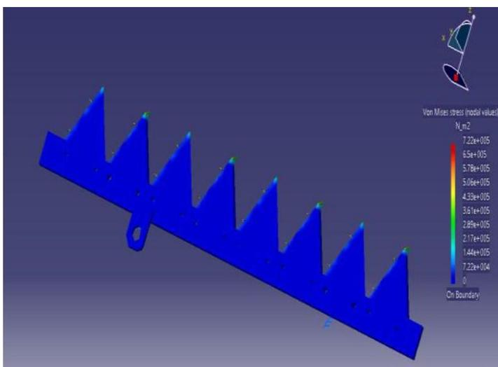
**Fig. 5** – Force Analysis on Cutter Blade
