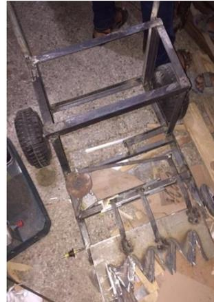
Fig. 3 – Assembly of Frame, Cutter and Wheels
