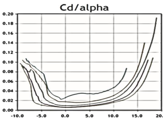
Fig.3 Coefficient of drag characteristics
