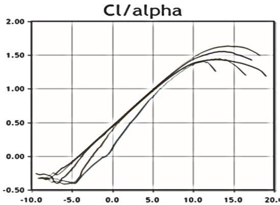
Fig.2 Coefficient of lift characteristics
