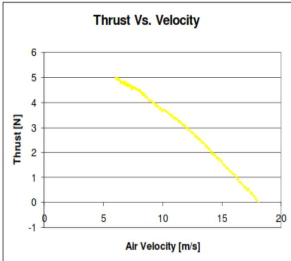
Fig .6 15"x10" Propeller. Thrust Vs. Velocity
