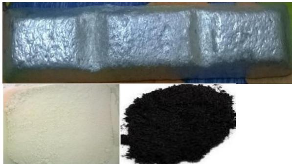
**Fig.1** Aluminum 7075 alloy ingot, TiO<sub>2</sub> powder and Graphene Oxide powder
