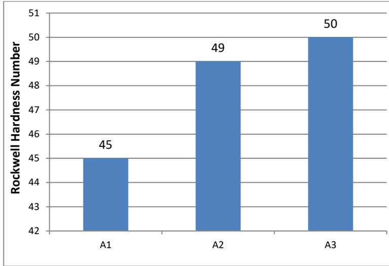
**Fig.3** Rockwell hardness test results where A1: Al-10%TiO<sub>2</sub>-0.5%GO, A2: Al-10%TiO<sub>2</sub>-0.75%GO, A3: Al-10%TiO<sub>2</sub>-1.0 %GO
