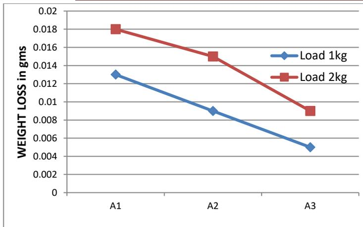
**Fig.6** Comparison of weight loss with composite specimens at various load conditions
