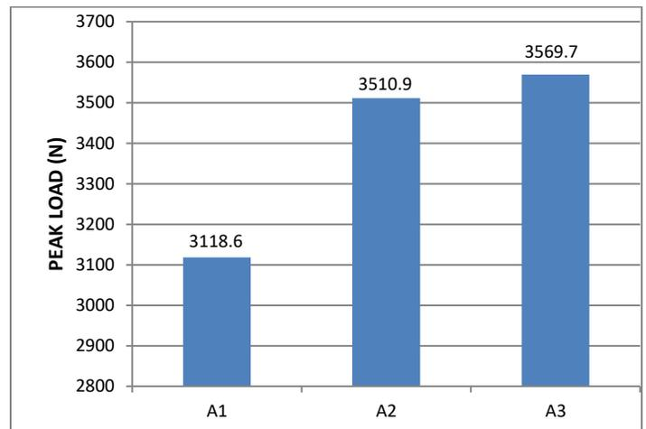
**Fig. 5** Variation of peak load with composite specimens
