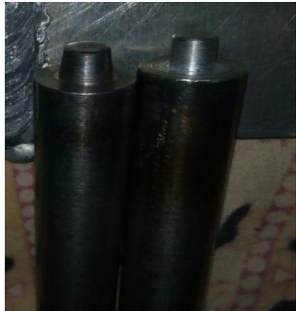
**Fig. 2** Tool Snapshot: 1) Tapered (left) 2) Cylindrical (right)
