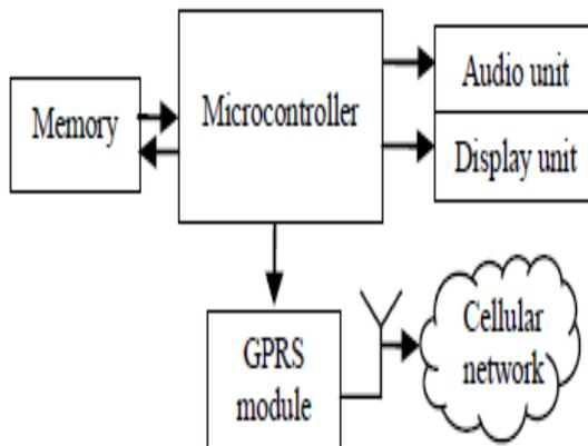
Fig.2 Station Unit Block Diagram
