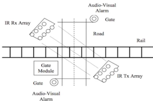
**Fig. 1:** Block diagram of Indian railway gate crossing.
