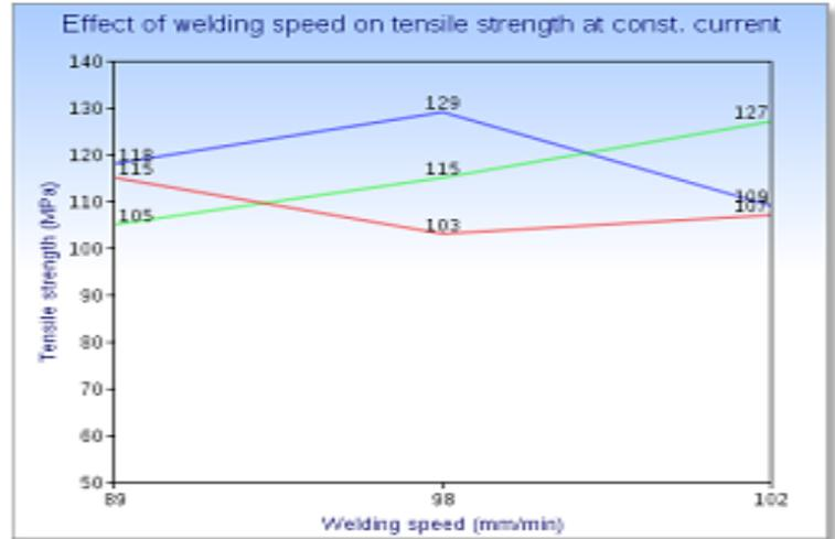
Fig. 3- Effect of welding speed on tensile strength
