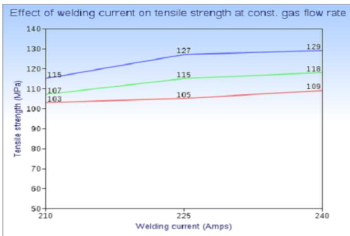
Fig.2- Effect of welding current on tensile strength
