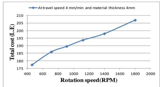
**Fig. 8** Relation between rotation speed and total cost (at material at at travel speed 4 mm/min and thickness 4mm)
