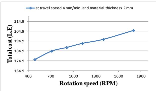
**Fig. 2** Relation between rotation speed and total cost (at travel speed 4 mm/min and material thickness 2mm)
