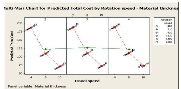
Fig. 18 Multi-Vari chart for predicted total cost by rotation speed, material thickness and travels speed
