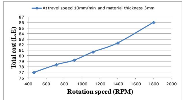
**Fig. 7** Relation between rotation speed and total cost (at at travel speed 10 mm/min and material thickness 3mm)
