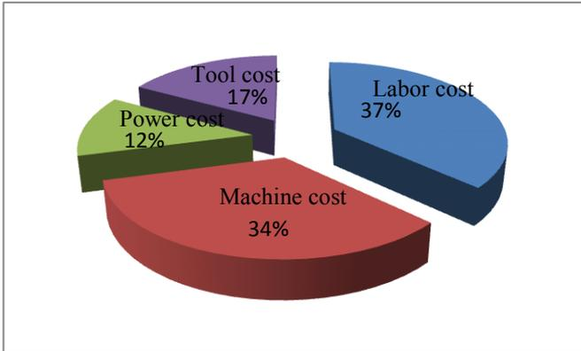
**Fig. 1** Shows the cost distribution for weld joint fabricated using FSW process.
