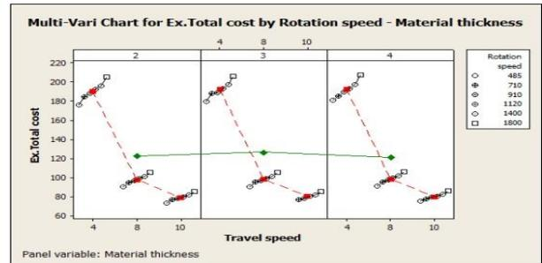
Fig.17 Multi-Vari chart for total cost by rotation speed, material thickness and travels speed
