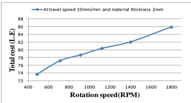
**Fig. 4** Relation between rotation speed and total cost (at travel speed 10 mm/min and material thickness 2mm)
