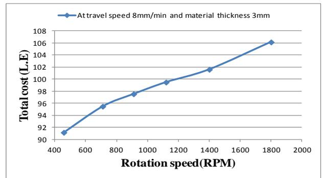
**Fig. 6** Relation between rotation speed and total cost (at at travel speed 8 mm/min and material thickness 3mm)
