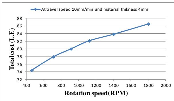
Fig. 10 Relation between rotation speed and total cost (at at travel speed 10 mm/min and material thickness 4mm)
