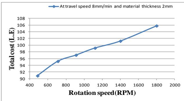
**Fig. 3** Relation between rotation speed and total cost (at travel speed 8 mm/min and material thickness 2mm)
