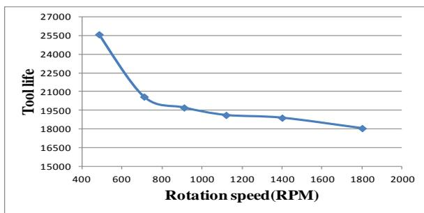
Fig. 11 Relation between rotation speed and tool life
