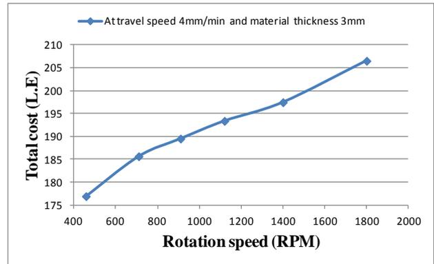
**Fig. 5** Relation between rotation speed and total cost (at at travel speed 4 mm/min and material thickness 3mm)
