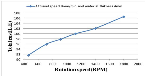
Fig. 9 Relation between rotation speed and total cost (at at travel speed 8 mm/min and material thickness 4mm)
