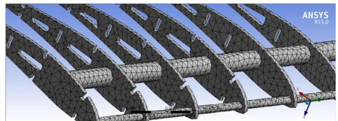
Fig.16 Successfully generated mesh
