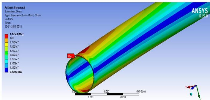
Fig.21 Equivalent Von-mises stress contours in spar
