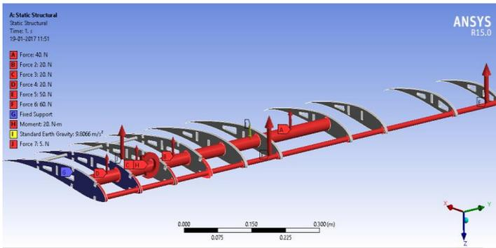
Fig.18 Force application on the wing
