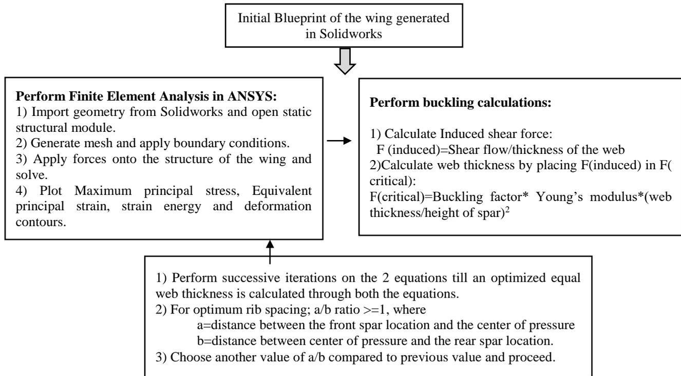
Fig.13 Structural optimization flowchart
