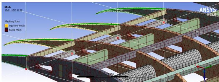
Fig.14 Failed & Obsolete Mesh (1<sup>st</sup> attempt)
