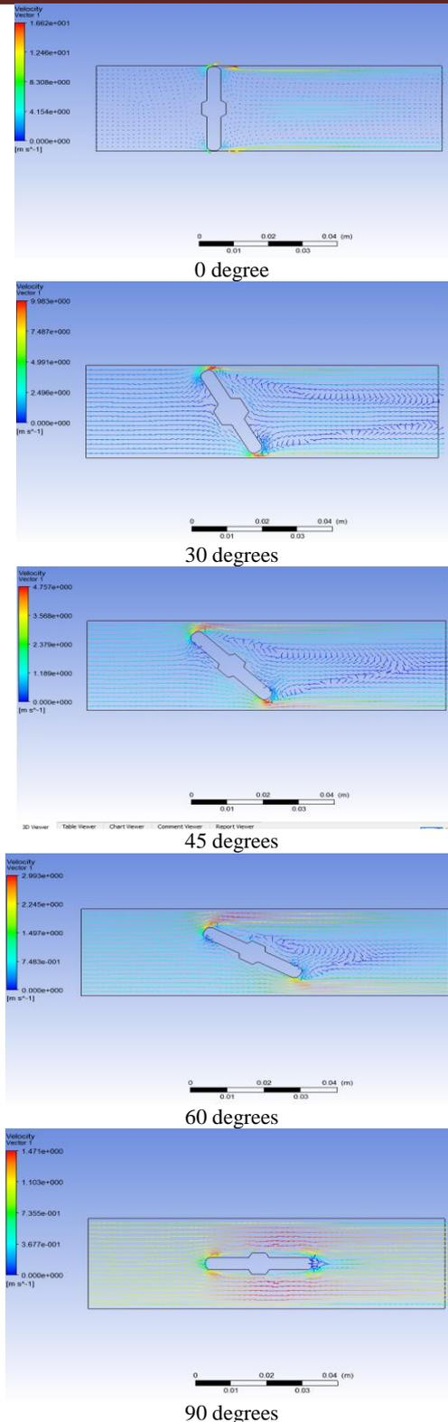
**Fig. 2** Velocity plots of the different throttle opening positions
