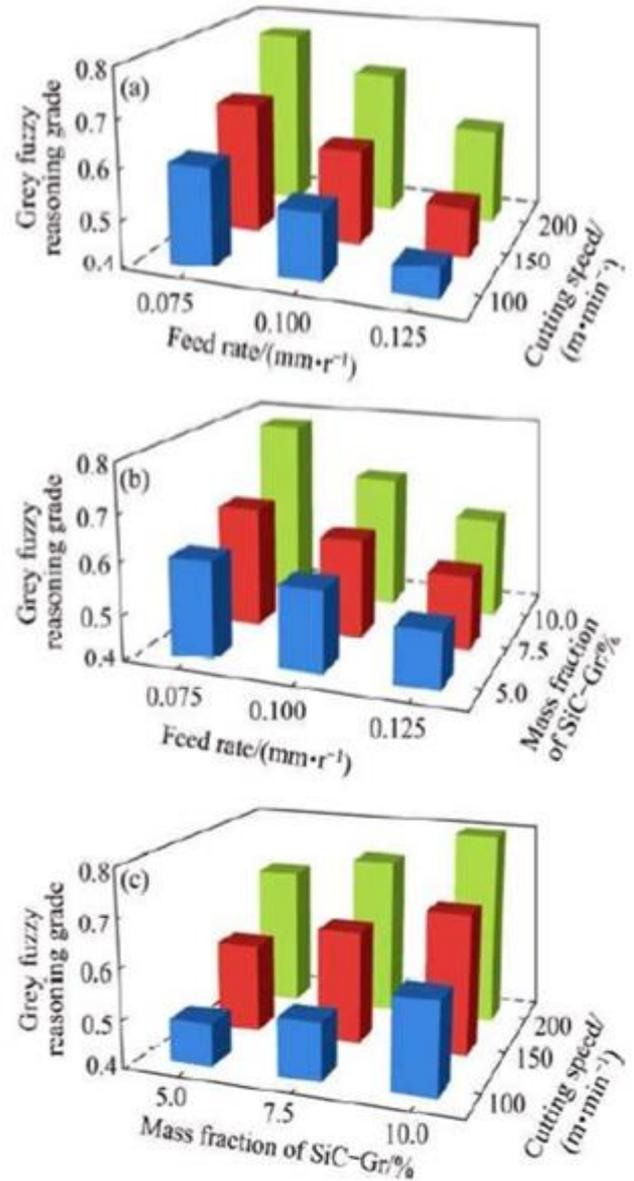
**Fig.9** Effect of Grey-fuzzy reasoning grade on machining parameters: (a) feed rate and cutting speed (b) feed rate and mass fraction of SiC-Gr (c) mass fraction of SiC-Gr and Cutting speed [15].
