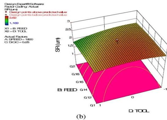
Fig.6 3-D graph (a) MRR (b) SR(surface roughness) [16]
