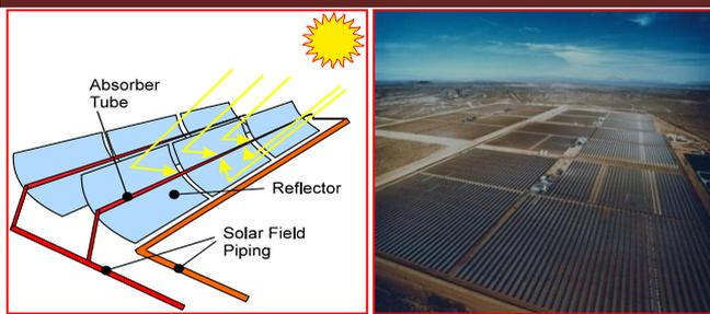
Fig.2 Solar Collector
