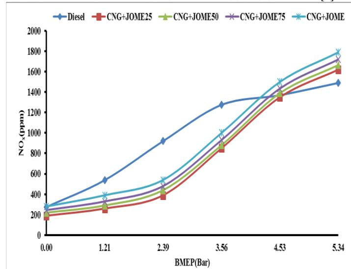
Fig. 8 Effect of BMEP on NOx
