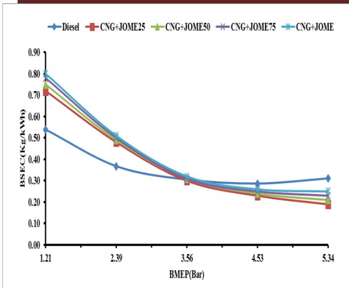
Fig.5 Brake specific energy consumption
