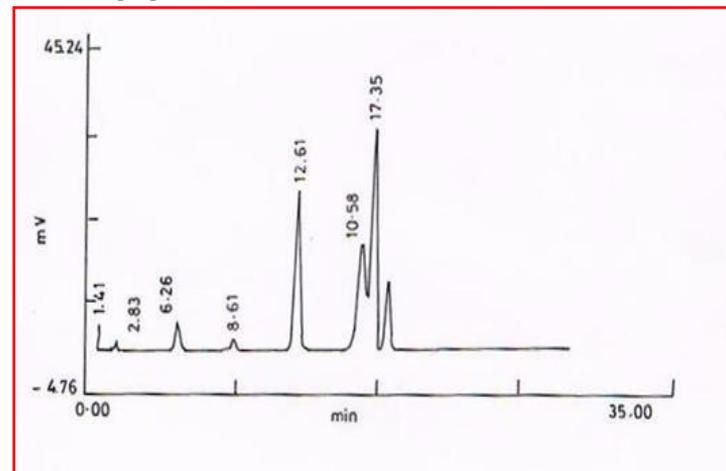
**Fig-3** Graph obtained from Gas Chromatograph for Jatropha oil biodiesel
