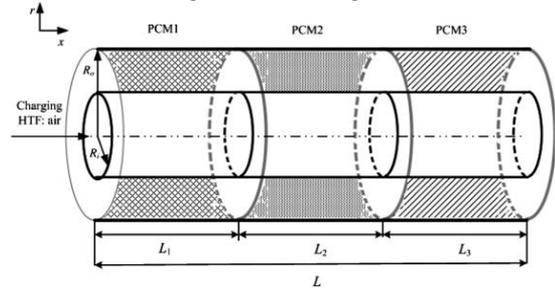
Fig. 4. Physical model of the LHTES unit with three PCMs
