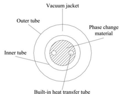
Fig. 7. Schematic diagram of thermal energy storage unit using Ba(OH)<sub>2</sub>.8H<sub>2</sub>O PCM.
