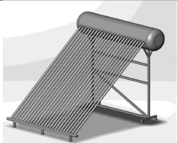
Fig. 2. Evacuated tube solar collector
