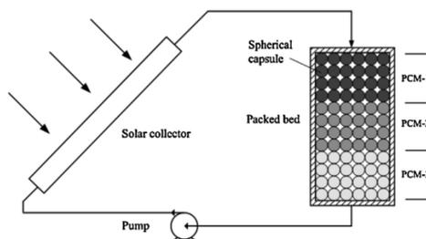
Fig. 6. Schematic diagram of the solar storage packed bed with multi PCM
