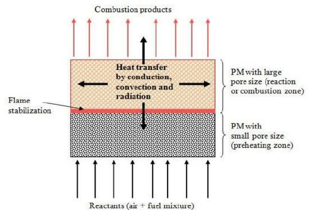
Fig. 1. Schematic diagram of two layer porous burner.
