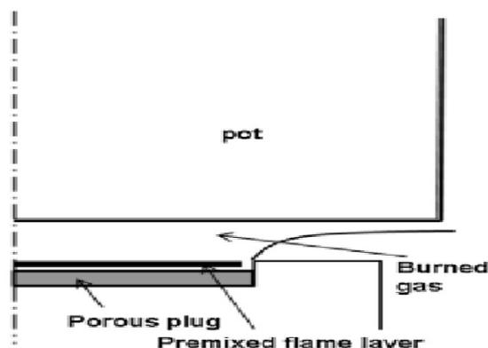
**Fig. 10.** The flat flame burner developed by Wu et al. (2014).
