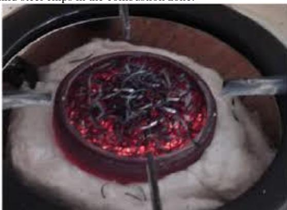
Fig.6. Porous burner studied by Pantangi et al. (2007).
