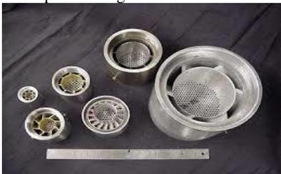
Fig. 3.Swirling flame burner proposed by S. Jugjai et al. (2001).
