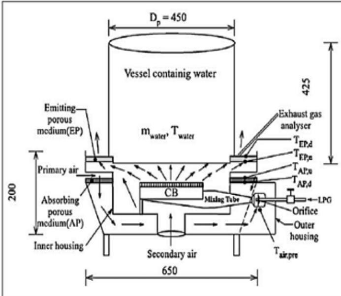
Fig. 2.PRRB Burner proposed by Jugjai and Sanitjai (1996).
