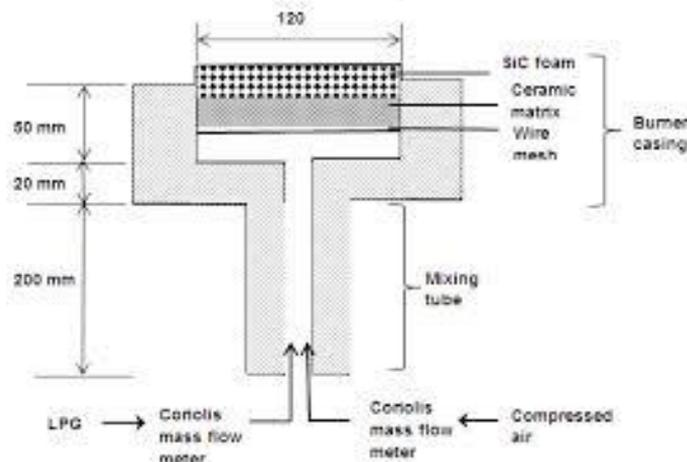
Fig. 7. The two-layer porous burner developed by Muthukumar and Shyamkumar (2013).
