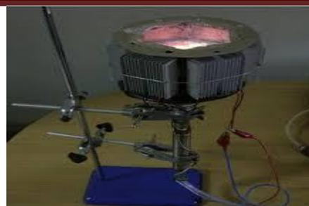
**Fig.9.** The micro cogeneration system developed by Ismail et al. (2013).
