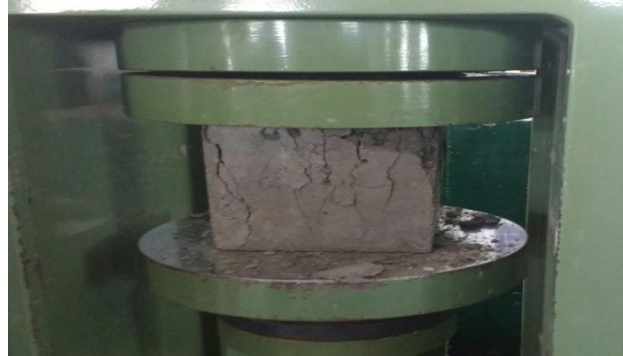
Figure 4 Compression test set up Table 6 Compressive strength of cubes (basic PET bottles fiber test)
