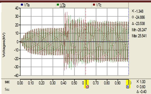
**Fig. 3** 13.8kV phase voltages of unloaded tertiary winding of 502 MVA Transformer with load rejection at 110kV Substation.
