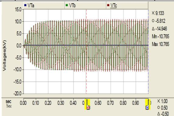
**Fig.4** 6.6kV phase voltages of unloaded tertiary winding of 73 MVA Transformer with LG fault at 13.8kV Switchgear.
