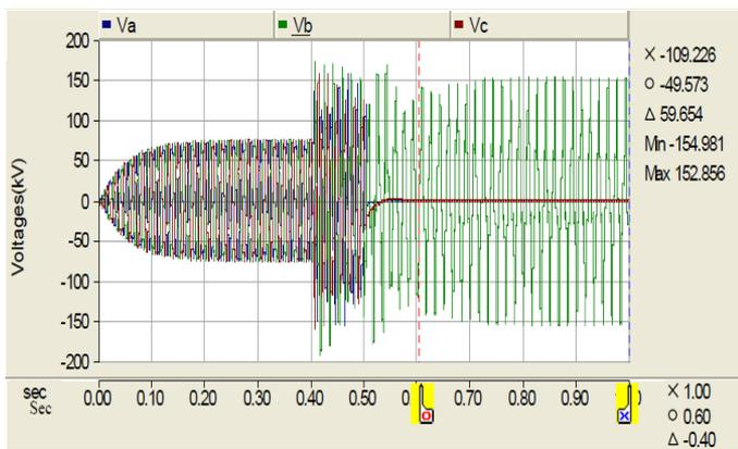
**Fig.1:** 110kV Phase voltages for load rejection and LLG fault at 110kV substation
