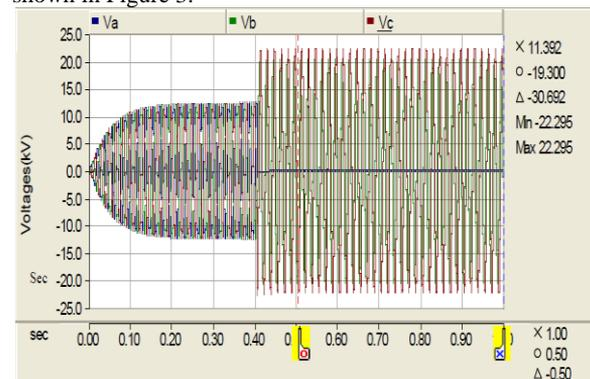
**Fig.2** 13.8kV Phase voltages at Al-Adel S/S for LG fault at Al-Adel 13.8kV Switchgear
