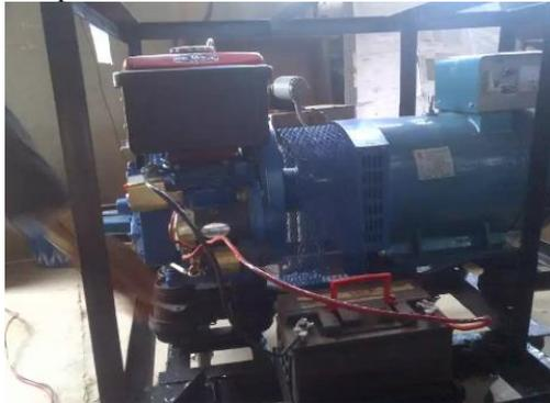
**Fig. 2:** 5kVA Diesel Generator Assembled
