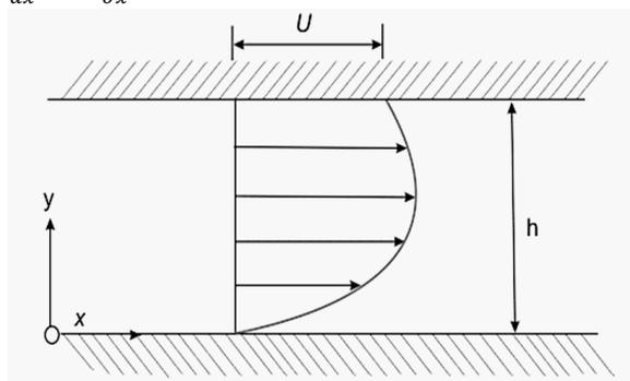
Fig 1 Couette Flow between two pipes
