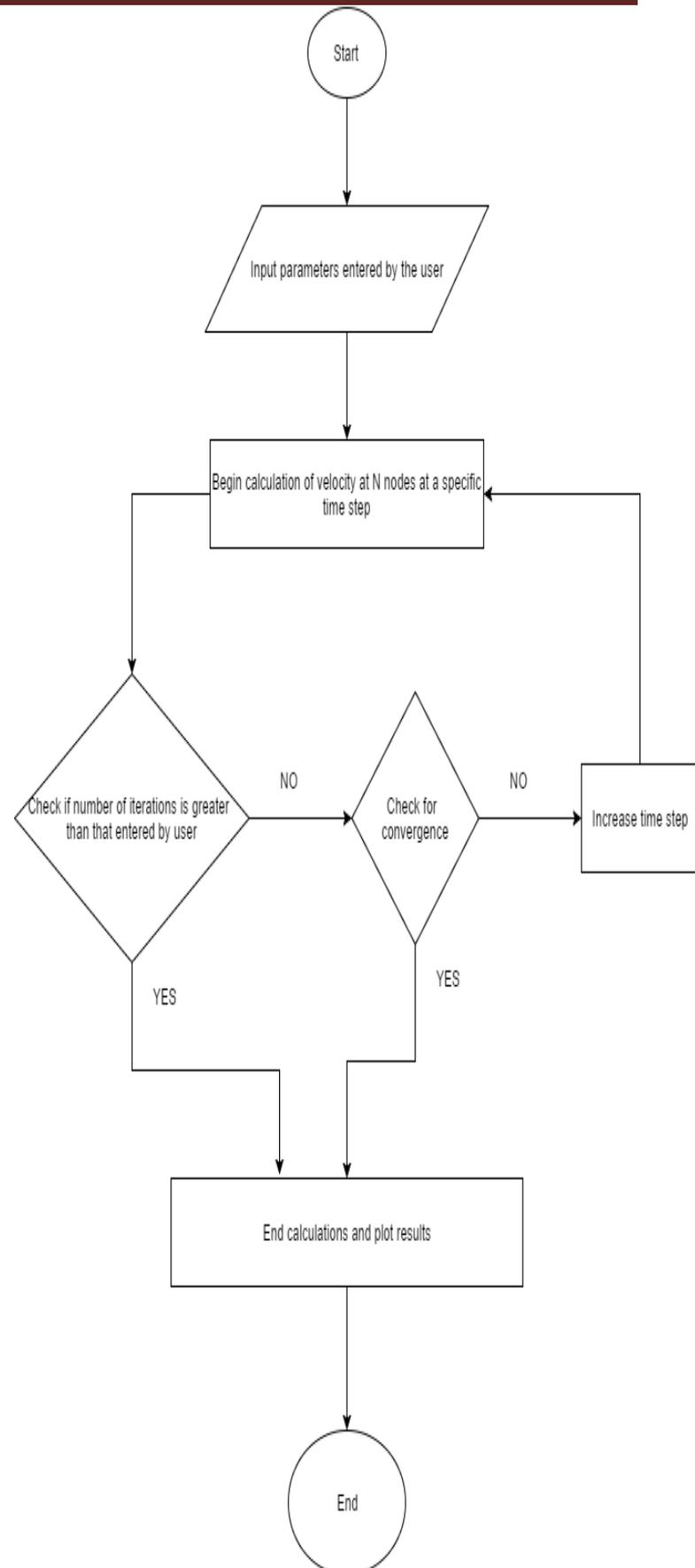
Fig 3 Algorithm used by the solver
