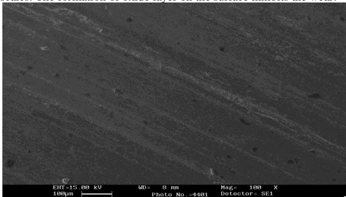
Fig. 2 (a): SEM Micrograph of worn surface of AISI D3 steel pin at speed 1.15 m/s
