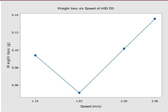
Fig. 1(a): Friction behaviour of AISI D3
