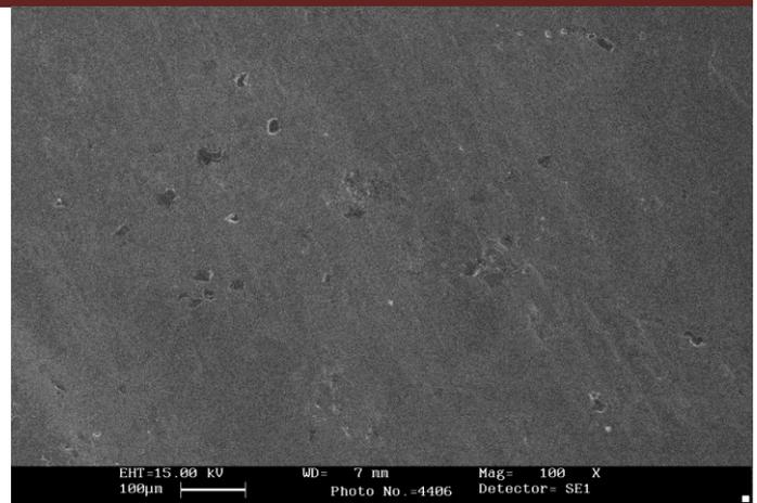
Fig. 2 (b) SEM Micrograph of worn surface of AISI D3 steel pin at speed 1.67 m/s
