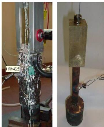
Fig. 5 Experimental set up dictating usage of heat pipe and cylindrical tank with thermoelectric modules.[4]
