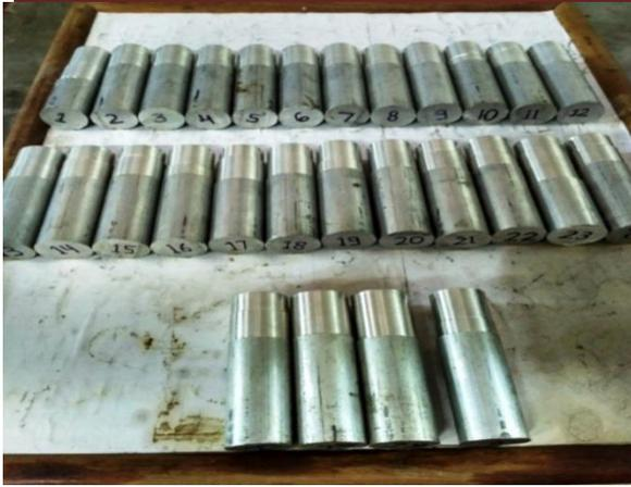
Fig. 2: AA6082 Workpiece after Turning
