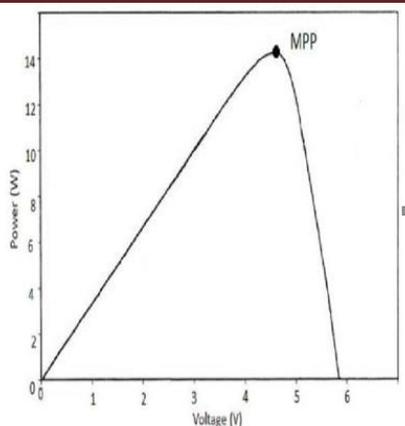
Fig 3: P-V curve of PV cell
