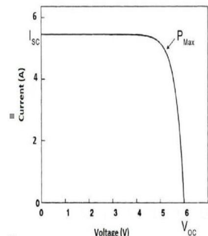
**Fig.2.** I-V curve of PV cell
