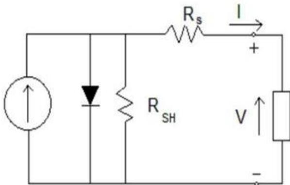
**Fig. 1:** Mathematical model of PV module
