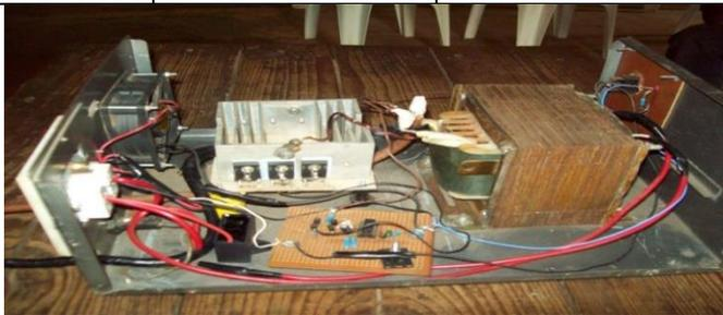
**Fig.2:** The Picture of the Assembled 0.75kVA Inverter
