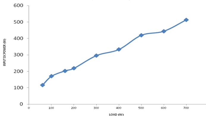
**Fig.3:** Input DC Power versus Load
