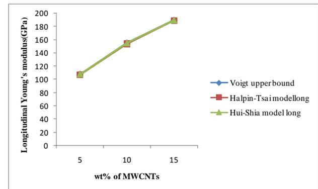
**Fig. 4:** Variation of longitudinal Young's modulus with wt% of MWCNTS
