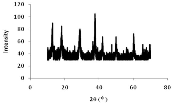
**Fig.3:** XRD pattern of 10 wt% MWCNTs/MnO<sub>2</sub>
