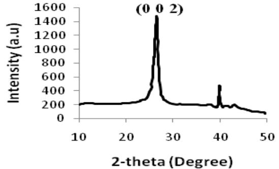
**Fig.2:** XRD Pattern of MWCNTs
