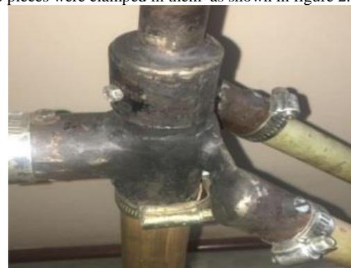
Fig. 2: The bush and clamp joining system
