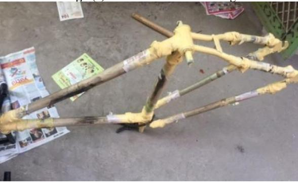
Fig.3(b): After coating the joints
