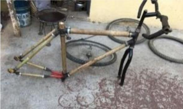
Fig.3(a): The frame before coating
