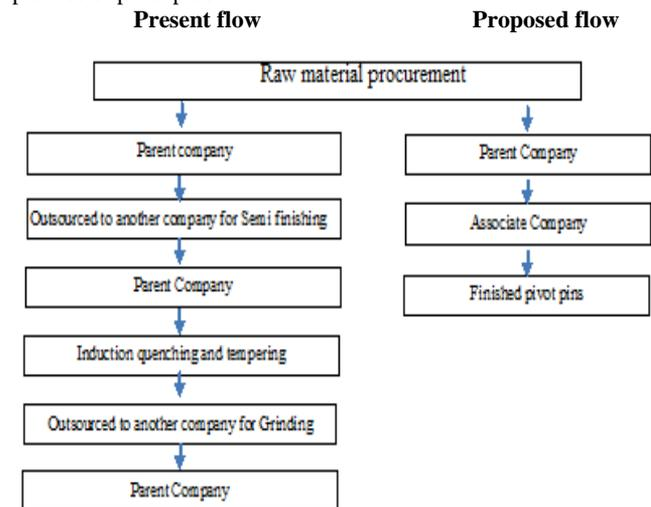
Fig. 1: Present and proposed flow process of pivot pins
