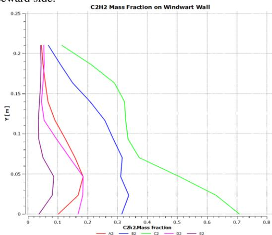
**Fig.9 (ii):** Pollutant mass fraction plots along sample lines on windward side.
