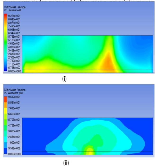
Fig. 6: Pollutant concentrations on (i) leeward wall and (ii) windward wall
