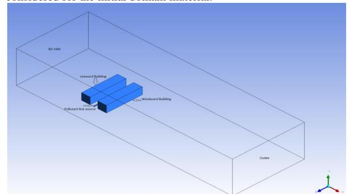
**Fig.1:** Three dimensional fluid domain and geometrical configuration
