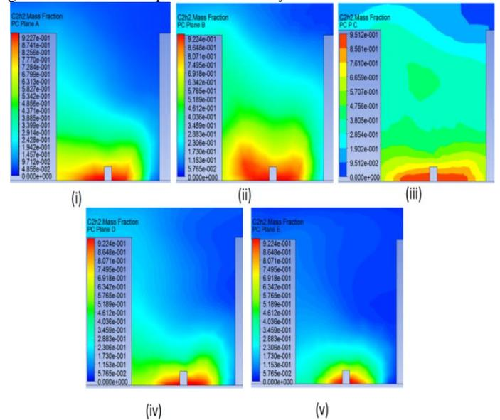
Fig. 5: Contours of pollutant mass fraction on (i) Plane A1A2, (ii) Plane B1B2, (iii) Plane C1C2, (iv) Plane D1D2, and (v) Plane E1E2
