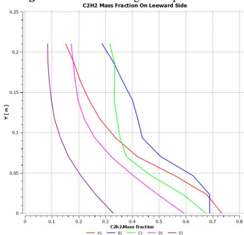
**Fig.9 (i):** Pollutant mass fraction plots along sample lines on leeward side.
