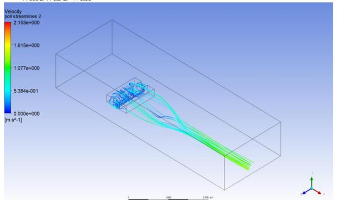
Fig.7: Streamlines of pollutant particles
