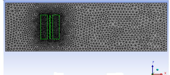
**Fig 2:** Bottom view of the grid generation of the fluid domain
