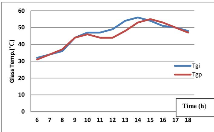
Fig.9: Variation of glass cover temperature with time
