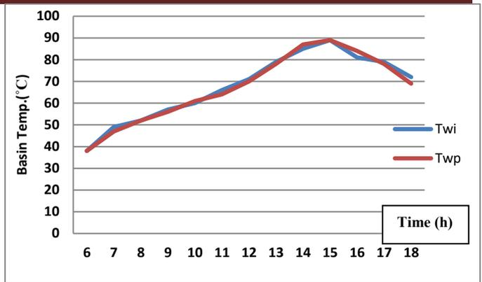
Fig. 10: Variation of basin temperature with time
