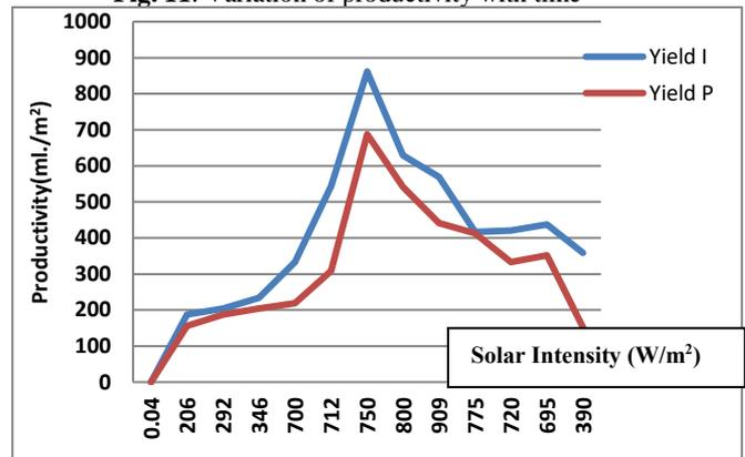
Fig. 12: Variation of productivity with solar intensity
