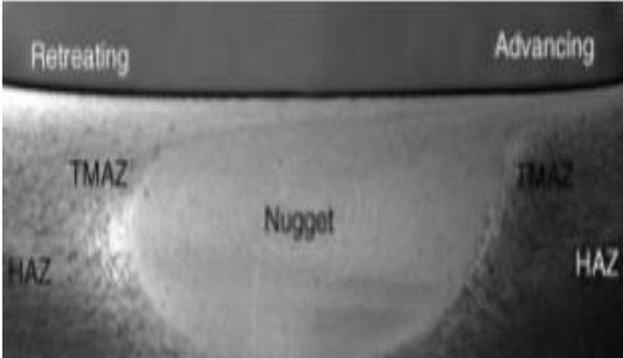
**Fig 4.** A macrograph showing various microstructural zones in FSP 7075Al-T651 (standard threaded pin, 400 rpm and 51 mm/min). [1]
