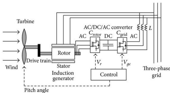
**Fig 1 :DFIG Based Wind Energy System Block Diagram**
