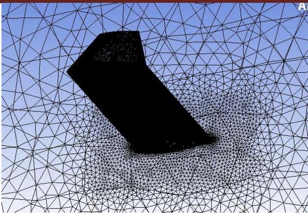
Fig. 9: Body sizing around elliptical winglet
