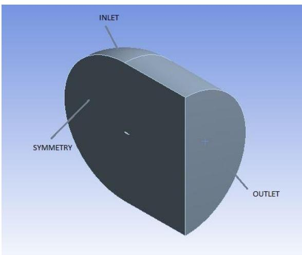
Fig. 11: Boundary conditions on flow field
