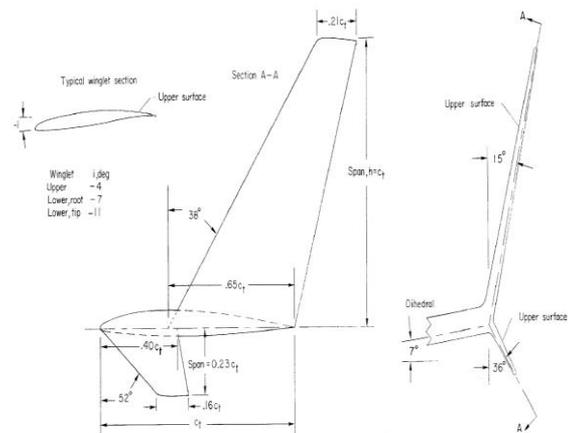
Fig.1: The winglet geometry used by Richard T. Whitcomb [1] in his research at NASA Langley wind tunnel
