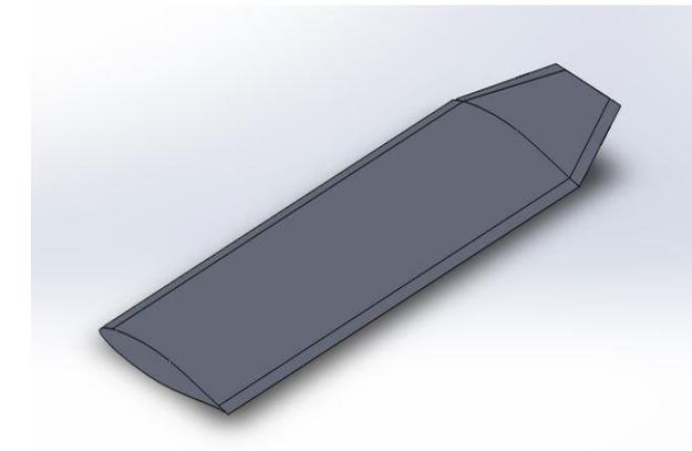
Fig. 4: Wing with Straight Winglet
