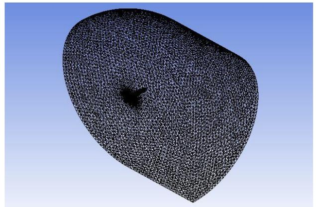
Fig. 8: Mesh for elliptical winglet
