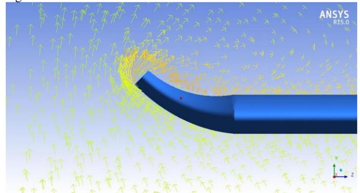
**Fig.17:** Vortex formation around elliptical winglet
