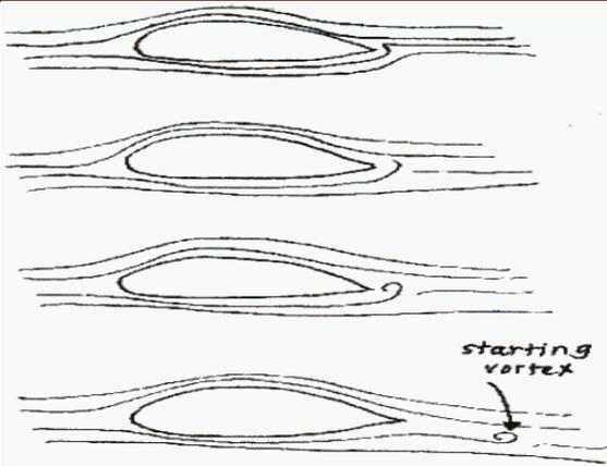
**Fig.14:** Circulation of air around wing conserving momentum [9]
