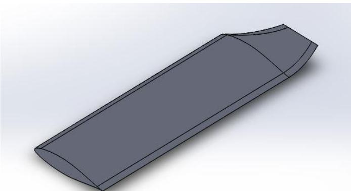
Fig.5: Wing with semi-circular winglet
