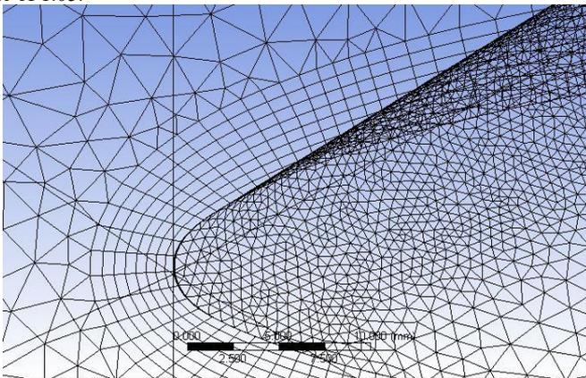
Fig. 10: Inflation layer around wing surface
