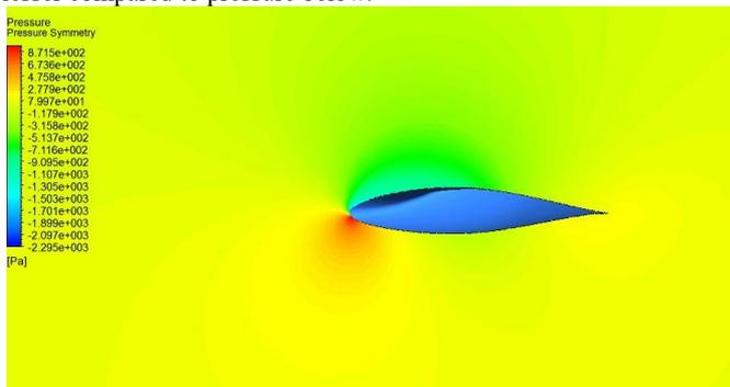
**Fig.16:** Pressure Contour on symmetry plane of elliptical winglet
