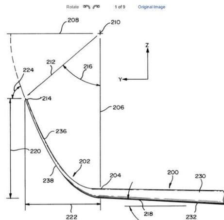
Fig. 7: Winglet shape Boeing patent US6484968 [8]
