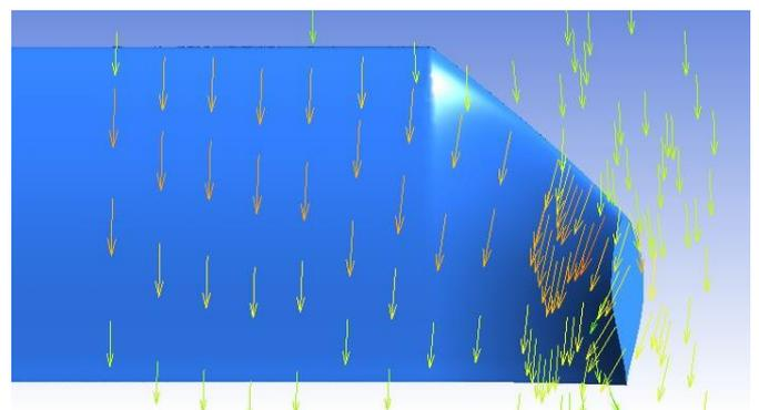
**Fig.18:** Direction of relative wind in vicinity of winglet surface
