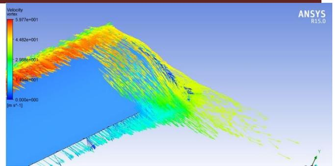
**Fig. 12:** Vortex formation on wing without winglet
