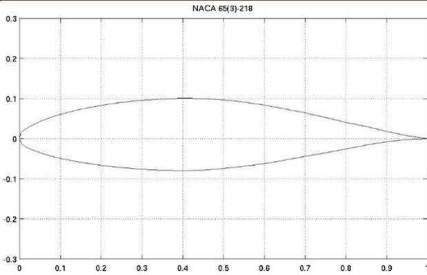
Fig. 2: Profile of NACA 65(3)218
