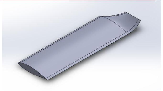
Fig. 6: Wing with elliptical winglet
