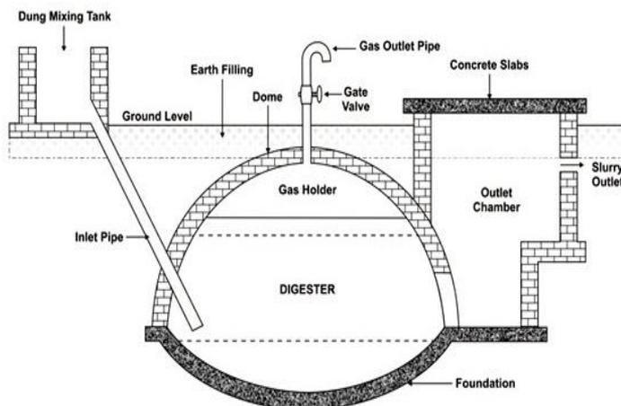
Fig. 4: Schematic diagram of a Deenbandhu biogas plant
