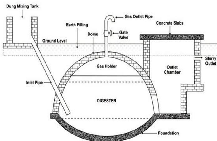
Fig. 4: Schematic diagram of a Deenbandhu biogas plant
