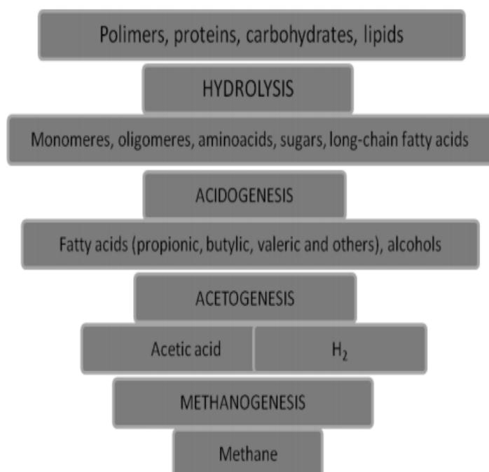
Fig. 1- Typical representation of anaerobic of complex substrates to biogas
