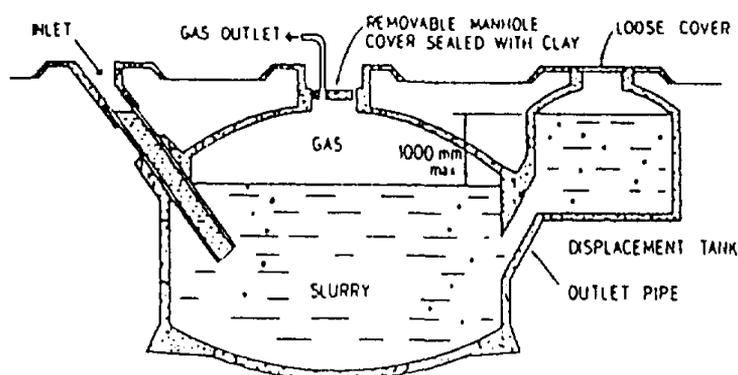
Fig.2- Schematic diagram of a KVIC biogas plant
