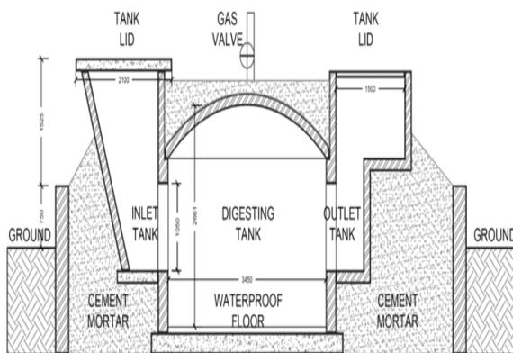
Fig. 3- Schematic diagram of a Janata biogas plant
