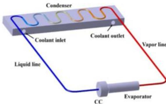
**Fig.2:** Loop heat pipe system
