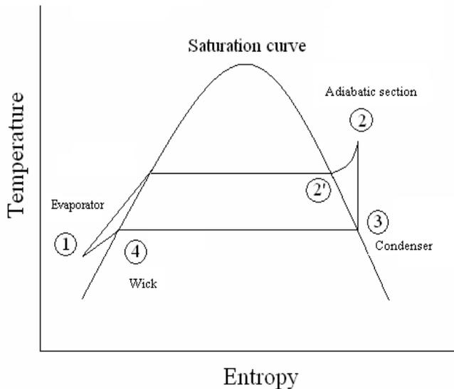
**Fig.1:** T-S diagram for a heat pipe [21]
